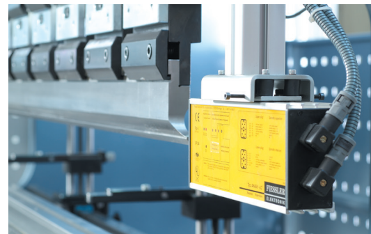
Ce Laser Safety System
